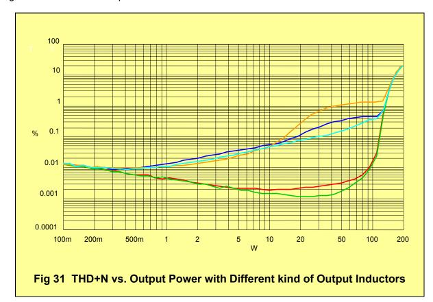
Fig 31 demonstrates THD performance difference with various inductors.
